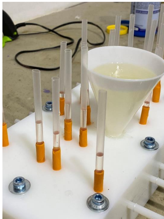
Figure 25: The leg mold after pouring.
