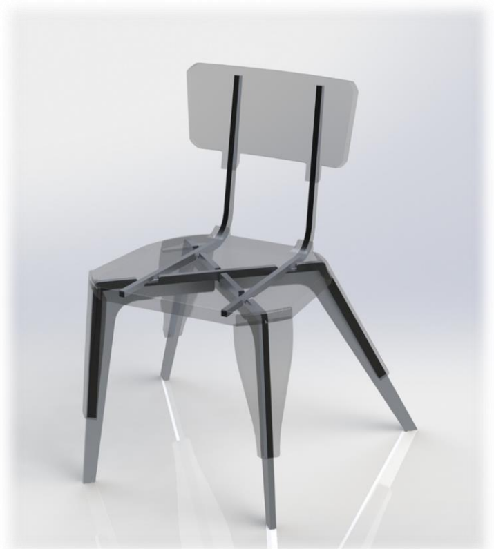
Figure 18: Pivoting to an aluminum frame.
