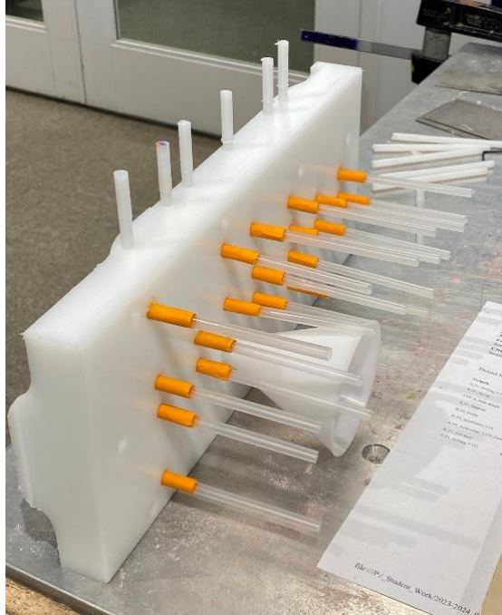
Figure 24: Inserting mold cores, risers, and pour cup into the leg mold.
