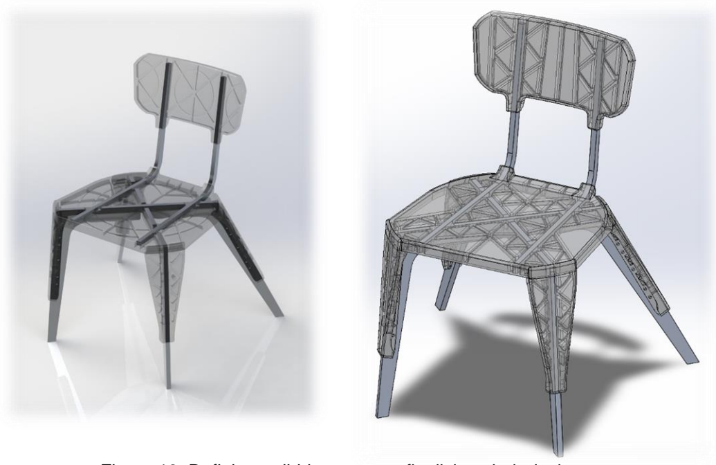
Figure 19: Defining a ribbing system; finalizing chair design.
