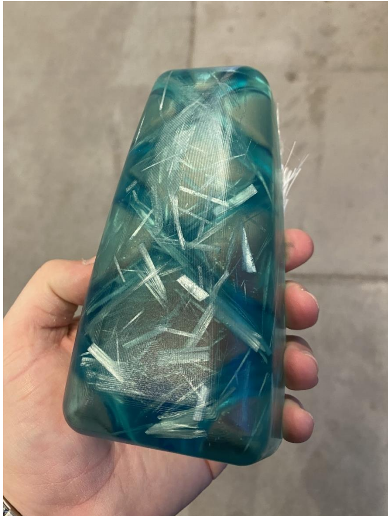
Figure 23: A fiberglass-insert pour from the process test mold.
