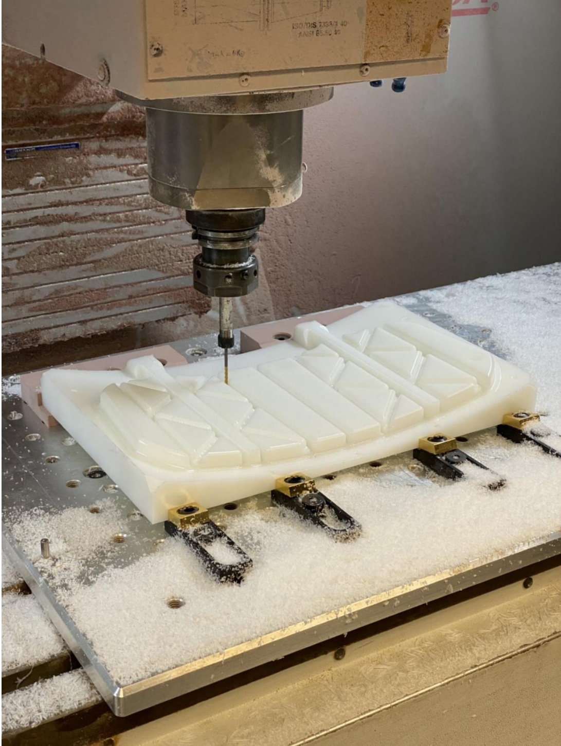
Figure 26: Machining the seat back mold.
