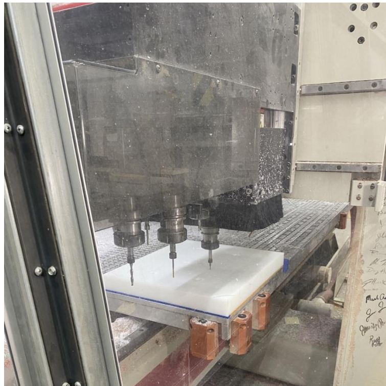
Figure 28: Machining the seat pan mold.
