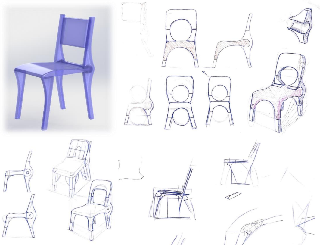
Figure 16: Further developing a plastic chair assembly.
